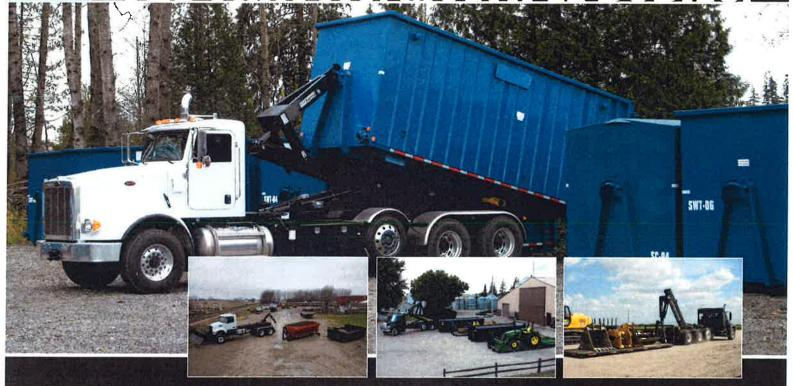
Stellar Industries provides the largest line of hydraulic hooklift hoists in North America. With both articulating tilt and sliding jib hooklifts, Stellar offers nearly fifty different models covering a wide range of capacities and body sizes.
