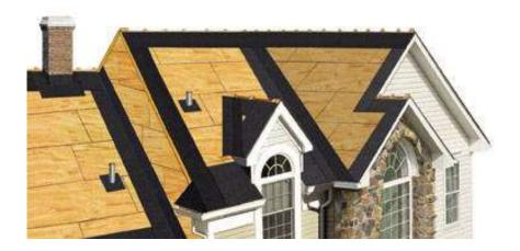
Ice and water shield is required for any roof over conditioned space. Ice and water shield shall extend from the eaves' edge to a point at least 24 inches inside the exterior wall line of the building. Ice and water shield shall be installed beneath the shingles in any valley, around chimneys, and over dormers. **R905.1.2**
